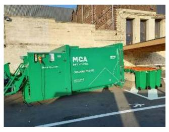
When the filled 140 litre containers collected from customers arrive back at the MCA Recycling site, they are taken to a central point and are emptied out (liners included) into MCA Recycling's own 16 tonne sealed organic compactor.
